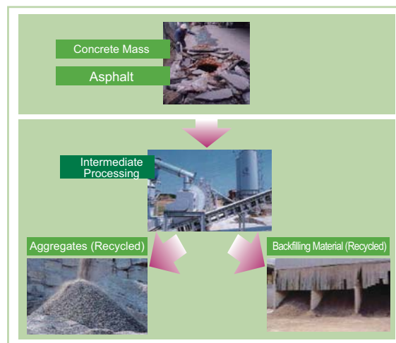
Figure 17: Flow of Industrial Waste Disposal in Civil Engineering Works
